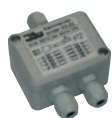
Terminal box VD-22, for universal application as a connecting box to take cross-sections 0.14...1.5 mm 2 , max. 48VAC Art. No. 80212
